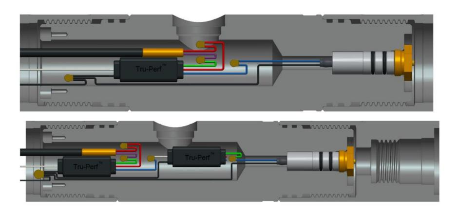
**Explosives must be resistorized (~50ohm)**
